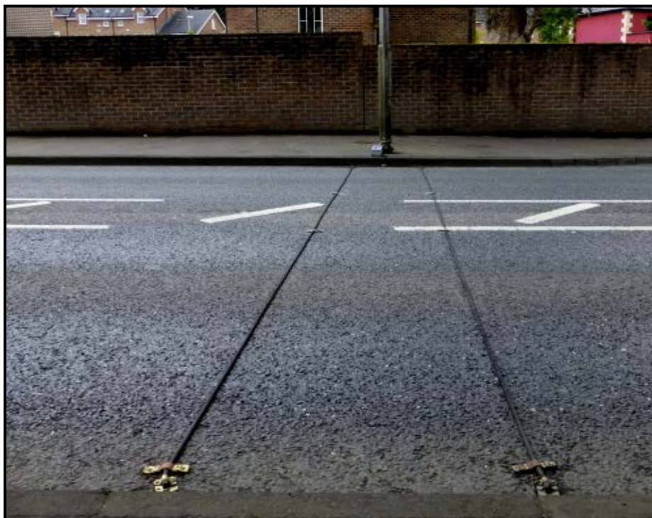
Figure 13.31 – Method of Data Collection on the Location of the ATCs
