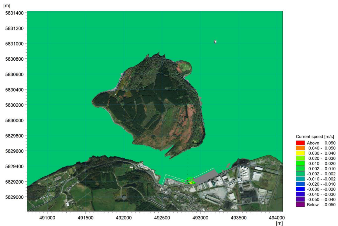
Figure 12.25 Difference in peak spring ebb current velocity Foynes Island – Proposed development minus existing
