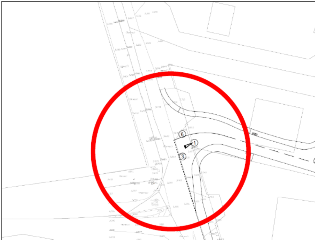
Figure 3.2: Proposed Staggered Priority Junction Arrangement on Main Port Access Road (Source: RPS drawing Proposed Road Markings – Sheet 1 of 4, ref: H0548-RPS-XX-00-DR-HE-110-02).
